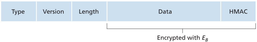
Figure 8.26 ♦ Record format for TLS
